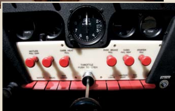
The instrument panel has a solid period feel, with a few custom additions, like the powder-coated piano switches at the center panel, and the custom-engraved bone-colored plastic panel. Detail at right.
