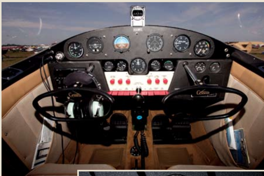
The instrument panel has a solid period feel, with a few custom additions, like the powder-coated piano switches at the center panel, and the custom-engraved bone-colored plastic panel. Detail at right.
