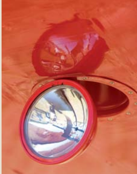
A Grimes retractable landing light is powered by a 60-amp alternator, the only major change to the accessory section of the newly overhauled Continental C-145.
